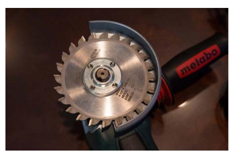
Officials at Austal modified this Metabo grinder by attaching a saw blade with teeth. Metabo Corp. explicitly warns against attaching this kind of blade because it can "create frequent kickback and loss of control."
