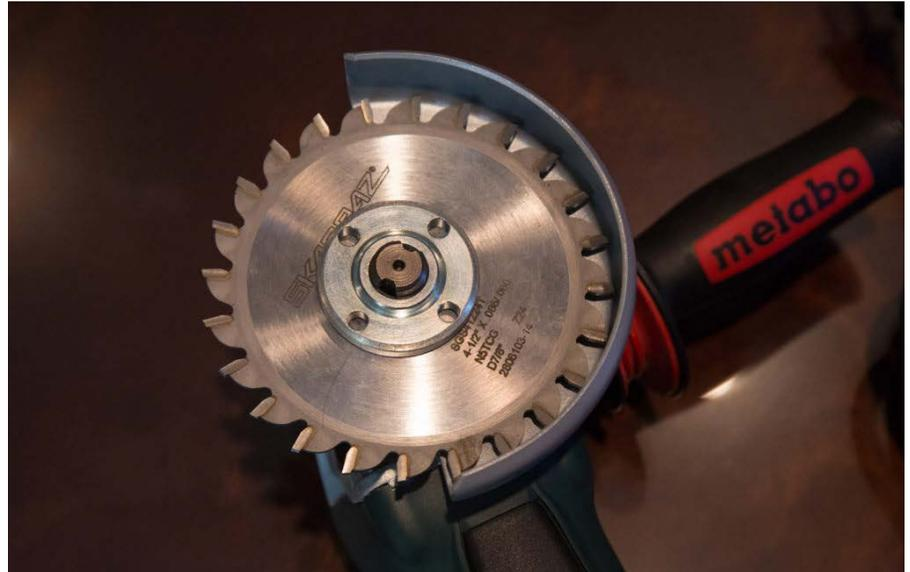
Officials at Austal modified this Metabo grinder by attaching a saw blade with teeth. Metabo Corp. explicitly warns against attaching this kind of blade because it can "create frequent kickback and loss of control."
